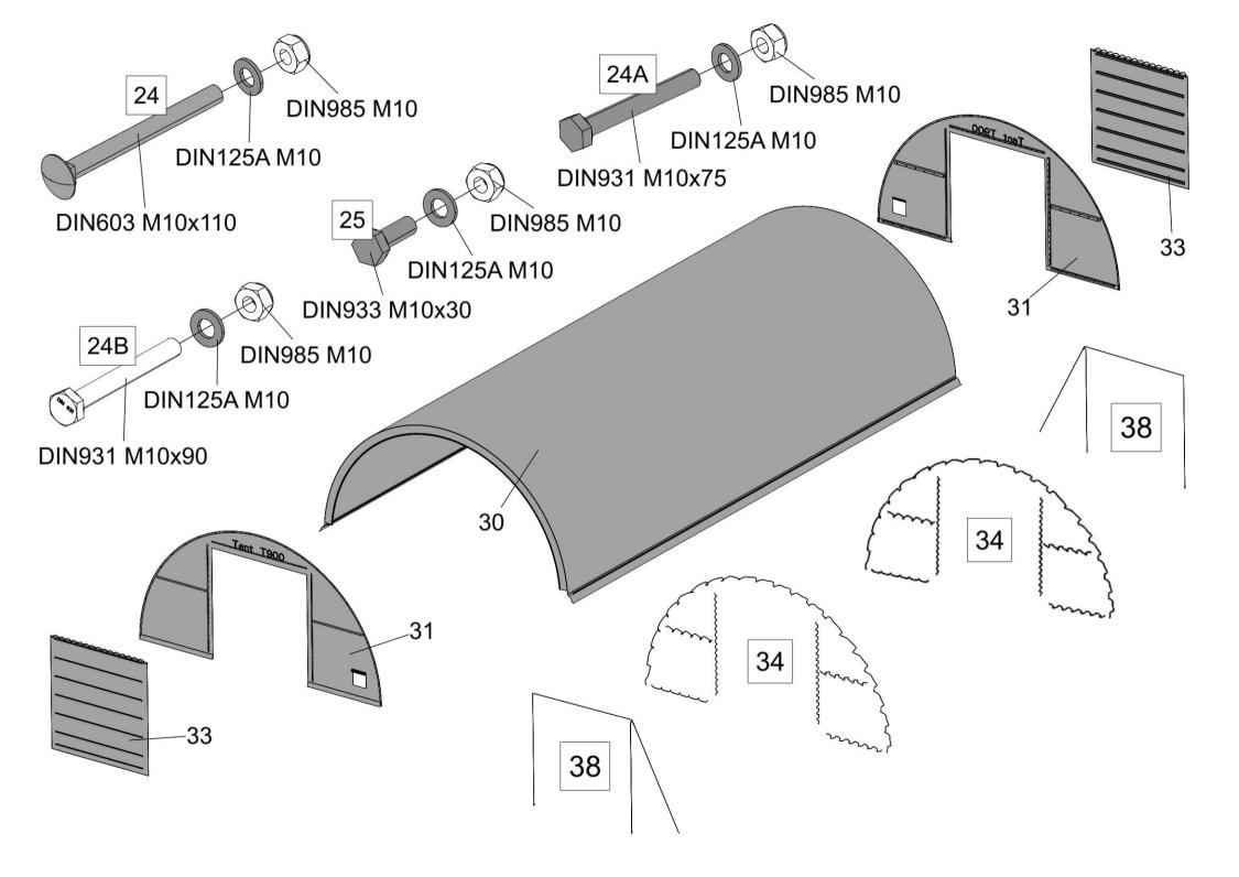
The tubes of the plates must be aligned in length and width.
