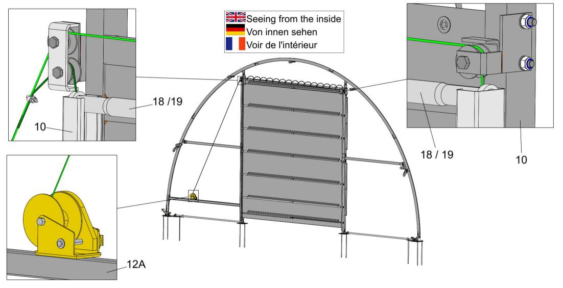
Place all "18 & 19" parts through the columns's rails "10", the rope on the corespondent wheels from "10" columns and in the end, connect the rope with the winch.
