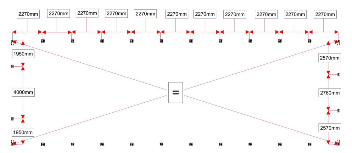
The measurements are taken between flanges's tubes, tubes which have to be align on length and width
