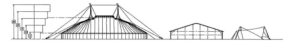
Figure 1 – Application of wind loads
